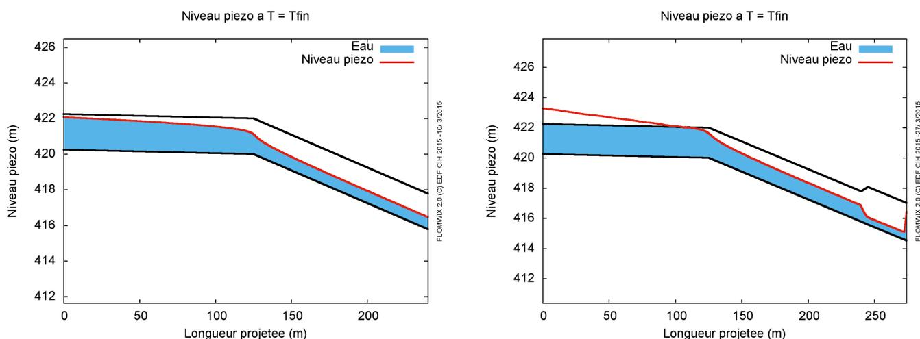
**Figure 7** : Conduite A : piezometric level versus horizontal length with a discharge of 4 m<sup>3</sup>/s (left) and a discharge of 7 m<sup>3</sup>/s (right)
