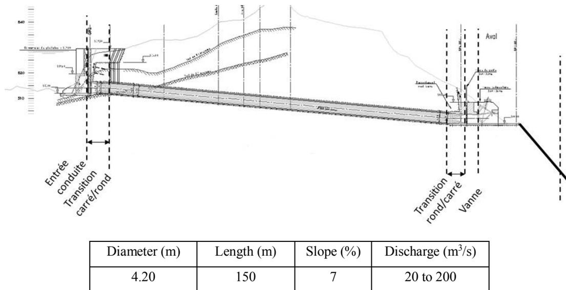
**Figure 8** : Scheme and characteristics of the tunnel
