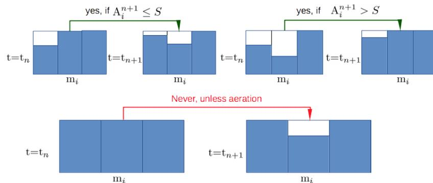
Figure 5: Update process of the state indicator
