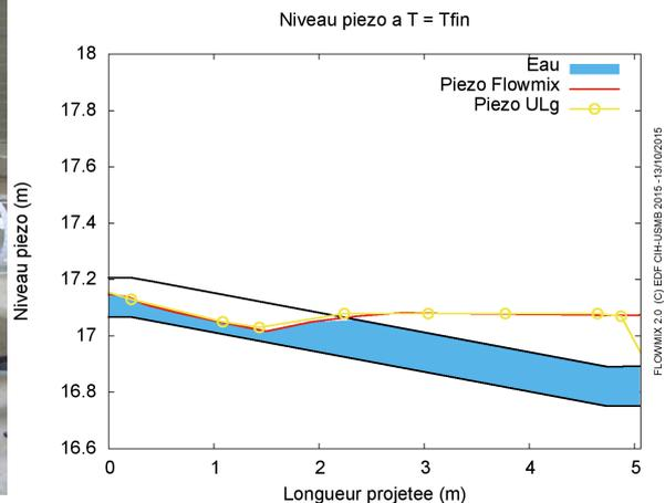
**Figure 10** : Free surface flow and pressurized flow on the model ( $25 \text{ m}^3/\text{s}$ , gate closed 20%) (left) and piezometric level versus horizontal length with comparison between FlowMix results and measurements on the model (right)
