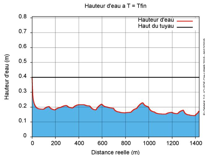
**Figure 13** : Water height versus real distance - FlowMix results
