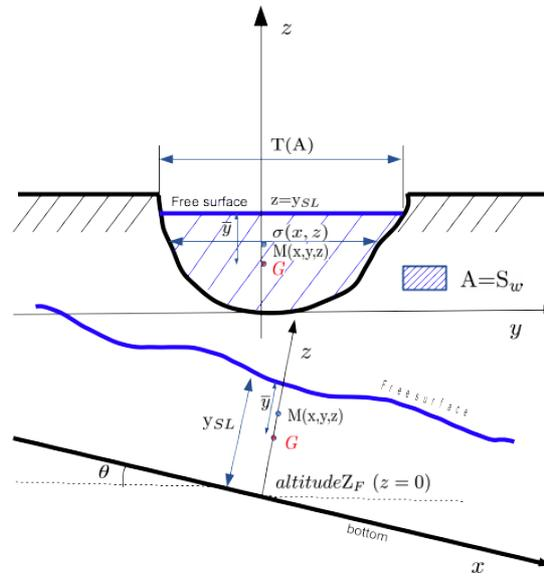
Figure 2: Free surface flow in a channel
